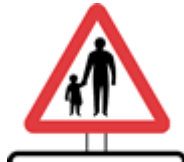
No footway for 400 yds Pedestrians in road ahead
