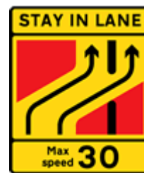
One lane crossover at contraflow road works
